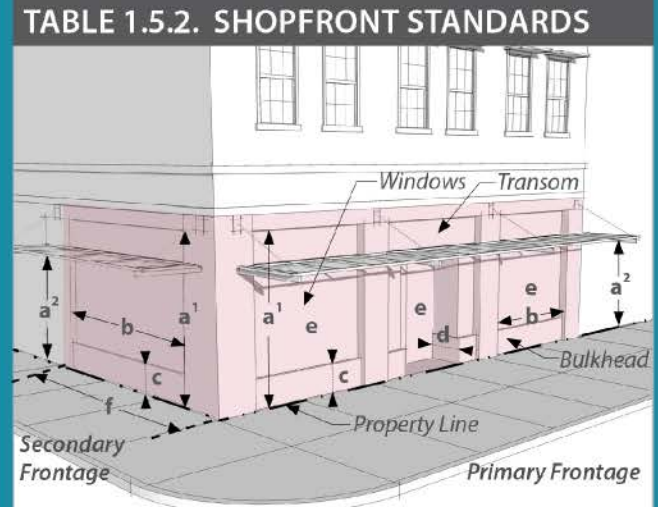
Shopfront diagram: Elements and dimensions, that when combined, make the Shopfront facade.
